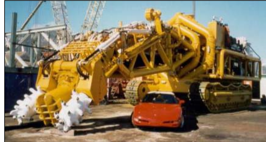
Second generation 200 ton offshore diamond mining machine, DeBeers, Namibia Courtesy Marine Minerals Pty
